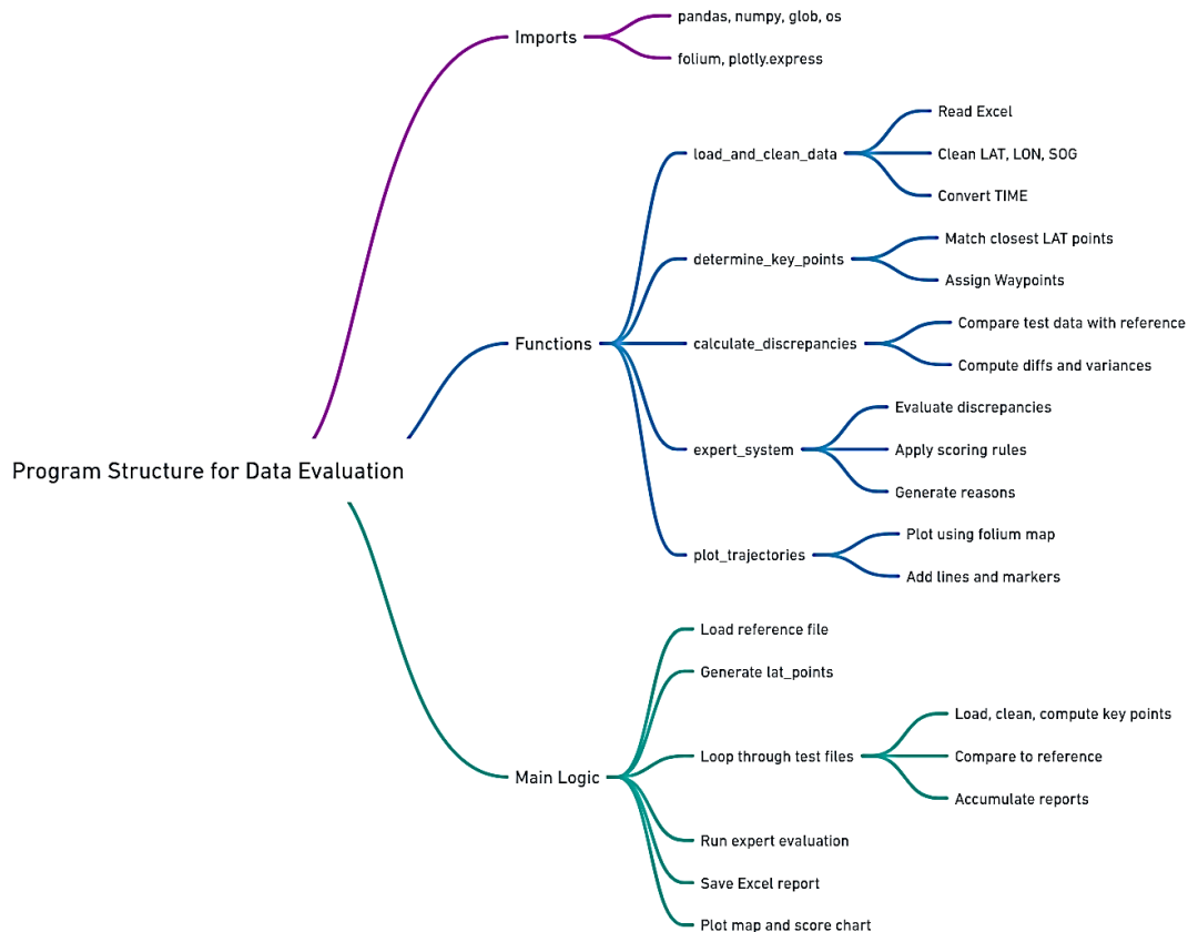
Fig. 2. Diagram of the Expert System for Analyzing Vessel Movement Trajectories
